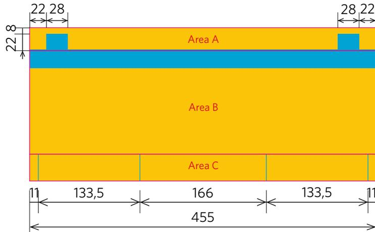
Traffic Board - first and last modules(only combined with the Quattro Board)
